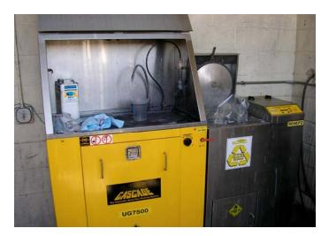
Figure 3-4. Typical Spray Gun Cleaning System
