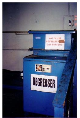
Figure 4-1. Typical Open Top Vapor Degreaser
