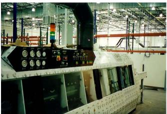
Figure 4-4. Conveyorized Printed Circuit Board Cleaning System
